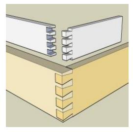
**Dovetail joints** - this is a strong method of joining two boards together at right angles, such as with drawer boxes. The ends of two boards or panels are notched with v-shaped cutouts that mesh with corresponding notches on the adjoining panel. If they're tight, these types of joints are considered very solid.
