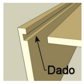
**Dado** - this is a groove that's cut into a board or panel that the edge of another board/panel can fit into. A good example is the sides and back of a cabinet drawer that are dadoed to accept the edges of the drawer bottom. It's a stronger way to 'capture' the drawer bottom than just gluing or nailing the drawer bottom edges to the side panels.
