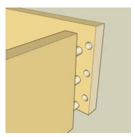
**Doweled joint** - this joinery technique uses round wood dowels (pegs) that are pressed and/or glued half way into holes drilled into one piece of wood. The protruding part of the dowel is then fit into holes drilled into the mating piece of wood. This method is another way to join the sides of drawers or cabinet boxes together.
